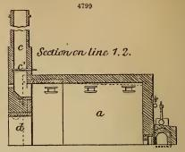
up clinkers; k k, flue-holes for spreading the. draught, which is carried through dampers  $b^1$  into the flue b, thence on to any other kiln as required.
